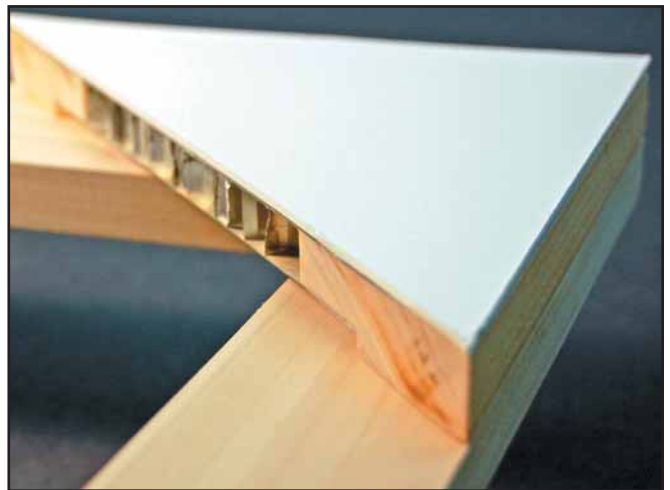
A honeycombed aluminum panel with 4-ply Museum board laminated to the surface was secured through the support strainer below, making a very rigid, solid platform to which the art was hinged.
