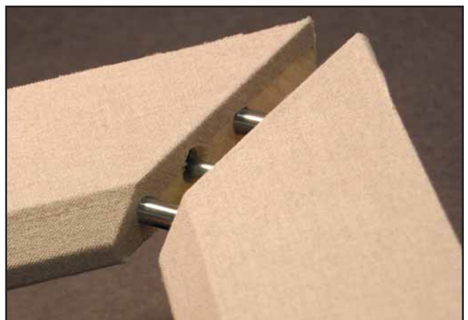
The linen-wrapped liner was also joined with an expansion bolt and two stainless steel dowels for extra strength.
